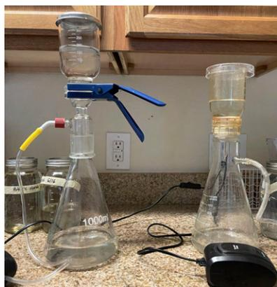
*Filter flasks attached to vacuum pumps.*
